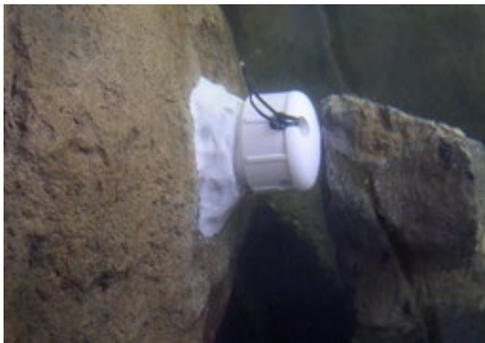
Sensor glued to an underwater rock to record hourly temperatures over extended time periods - Dan Isaak, U.S. Forest Service Photo.
